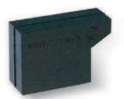
These vacuum switches feature reduced overall dimensions and give an electric signal when a certain adjustable vacuum level is reached. The pressure differential existing between the set maximum value and the value of reset of the rest signal is 50 ÷60 mbar and it is not adjustable.
