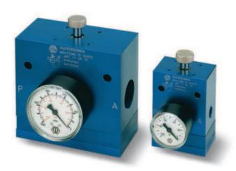
Vacuum regulators are used to adjust the pre-set vacuum level, keeping it constant (secondary vacuum), regardless of the capacity and the oscillations of the network vacuum level (primary vacuum).
