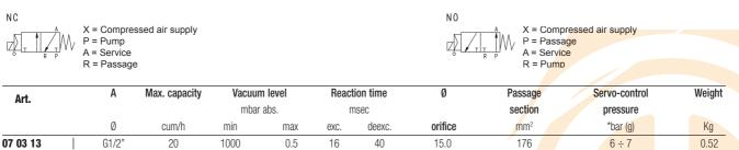
\* Add the letters LP to the article for servo-control pressure 4  $\div$  6 bar (g).
