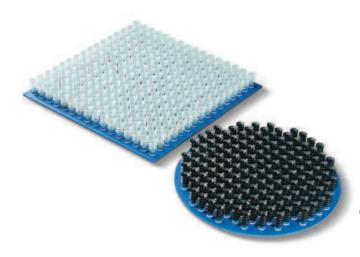
These suction plates provided with vacuum cups have been designed to ensure a better grip on uneven and very flexible surfaces (pasta or candy bags, blister or skin-film packs, thin cardboard boxes, etc.), which are difficult to grip with suction plates coated with foam rubber.
