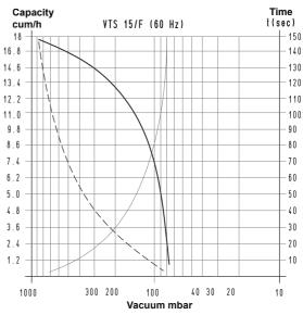
To calculate the emptying time of a volume  $V_1$ , apply the formula  $t_1 = \frac{1 \times V_1}{100}$
