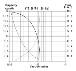
To calculate the emptying time of a volume  $V_1$ , apply the formula  $t_1 = \frac{t \times V_1}{100}$
