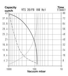
To calculate the emptying time of a volume  $V_1$ , apply the formula  $I_1 = \frac{1 \times V_1}{100}$
