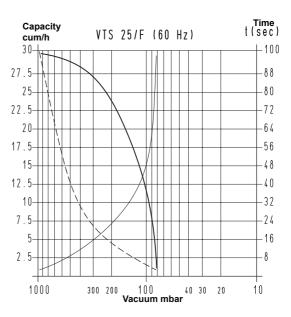
To calculate the emptying time of a volume  $V_1$ , apply the formula  $t_1 = \frac{t \times V_1}{100}$
