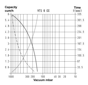
To calculate the emptying time of a volume  $V_1$ , apply the formula  $t_1 = \frac{1 \times V_1}{100}$
