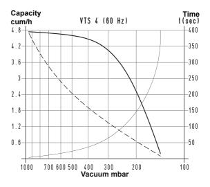
To calculate the emptying time of a volume  $V_1$ , apply the formula  $t_1 = \frac{t \times V_1}{100}$
