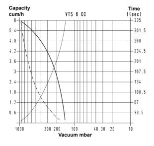
To calculate the emptying time of a volume V<sub>1</sub>, apply the formula  $t_1 = \frac{t \times V_1}{100}$
