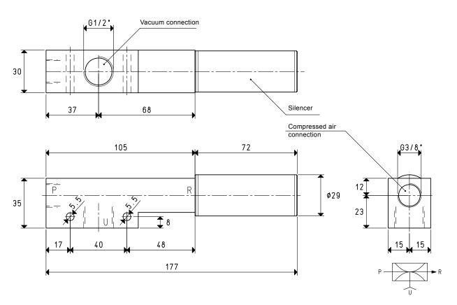
P=COMPRESSED AIR CONNECTION R=EXHAUST U=VACUUM CONNECTION 15 05 10 SX Art. Quantity of sucked air 12 12.2 12.5 cum/h -KPa 40 60 88 Max. vacuum level 400 **Final pressure** mbar ass 600 120 **Supply pressure** bar 2 3 3.4 Air consumption NI/s 3.7 5 5.5 Working temperature °C -20 / +80 **Noise level** dBA 63 Weight g 306 Spare parts Silencer SSX 3/8" art.
